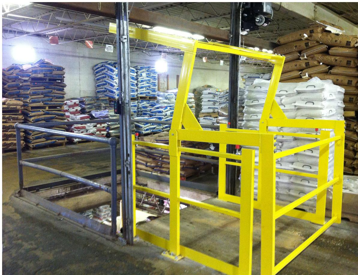
button opener. The operator still opens and closes the gate as required, however, if the gate is open in the access position for the 1st floor or the access position for the 2nd floor, the floor opening is secure for personnel.
